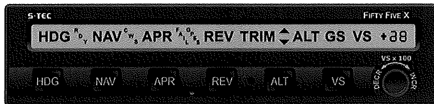
Fig. 2-1. AP Display, All Annunciations at Power-Up
