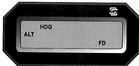
Fig. 3-41. Remote Annunciator Display, FD Mode Engaged
