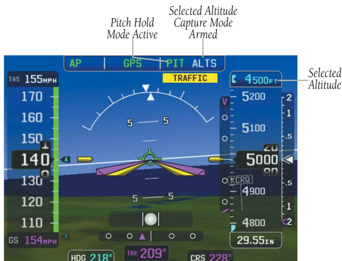
Pitch Hold & Selected Altitude Capture Modes
