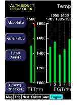
controller may automatically open the alternate induction door. If this occurs, then the ALTN INDUCT DOOR OPEN indicator displays on the Engine Page as long as the door is open. A message also displays in the message bar and on the Aux Main Page.
